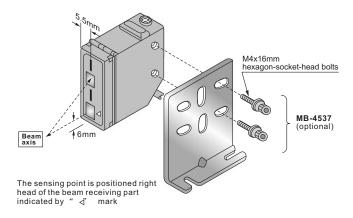
• Before installing the sensor, make sure of the travelling direction of objects to attitude of the sensor facing to
