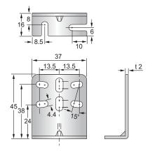
Material: Cold rolled carbon steel(spcc)
