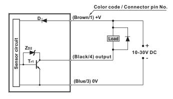
Symbol...D : Reverse polarity protection diode. ZD2: Surge absorption zener diode Tr1 : NPN output transistor.
