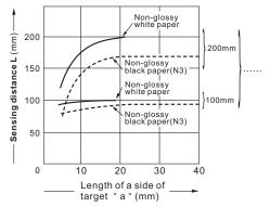
These curves show the values obtained against each target when the sensor is adjusted to have sensing distance of 100mm and 200mm against a target of 50x50 nonglossy white paper.
