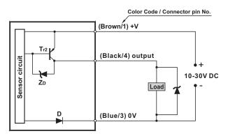
Symbol... D: Reverse supply polarity protection diode Zo: Surge absorption zener diode. Tr2: PNP output transistor.
